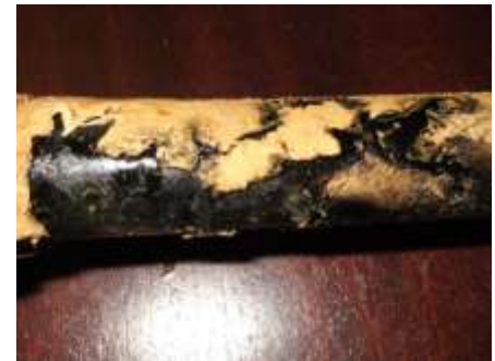
Sometimes, the product fails under test. The Yellow Stress Control Mastic in this test melted and flowed too easily under heavy load cycling conditions and caused tracking between the xlpe screen end and Connector. A new Tape was developed which subsequently tested out successfully.
